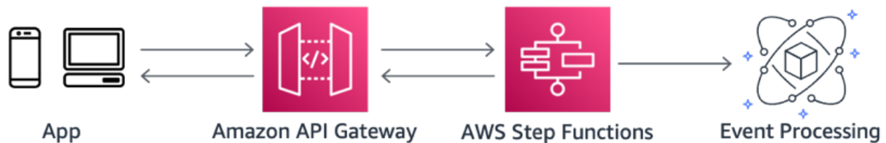
Figure 29: Asynchronous workflow with Step Functions state machines
