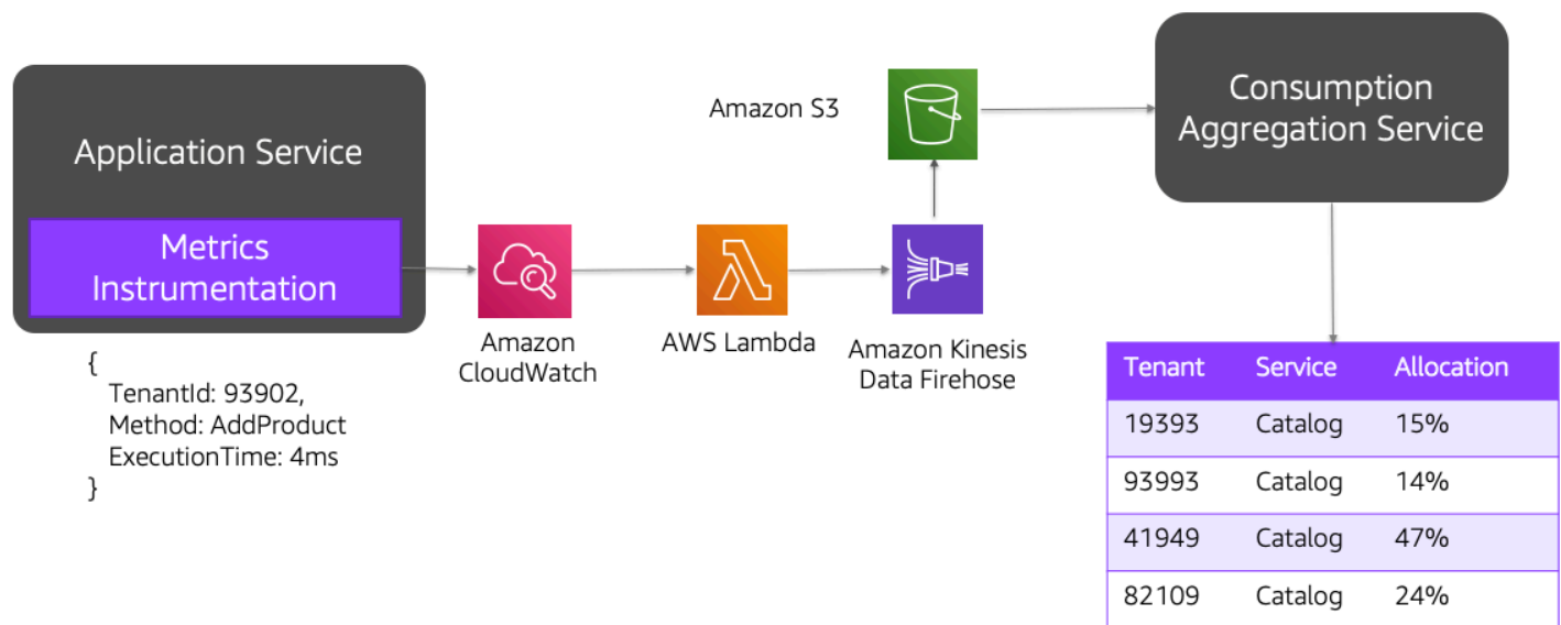
Figure 26: Instrumenting microservices with tenant consumption events
