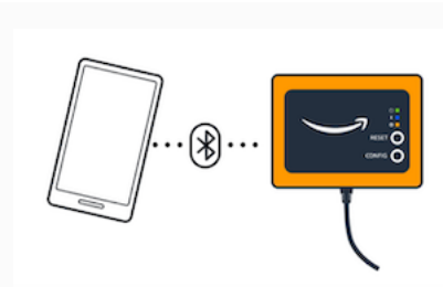
Bluetooth pairing with an Ethernet gateway.
